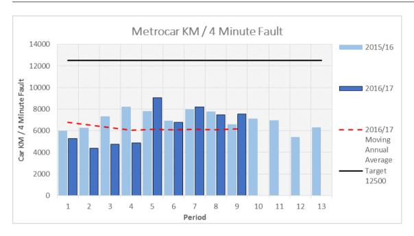
The current Metrocars were constructed in the late 1970s, and have served their purpose well. However despite undergoing two significant refurbishments, the fleet is coming to the end of its design life, with many components effectively life-expired, contributing to a very unstable operating environment. This is why Nexus plans to procure new rolling stock, intended to come into service in 2021. Discussions are underway with the government regarding the funding for new rolling stock.
